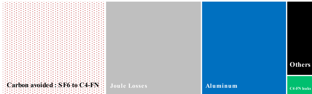
Figure 38: Carbon origins for a 145 kV C4-FN mixture GIS
