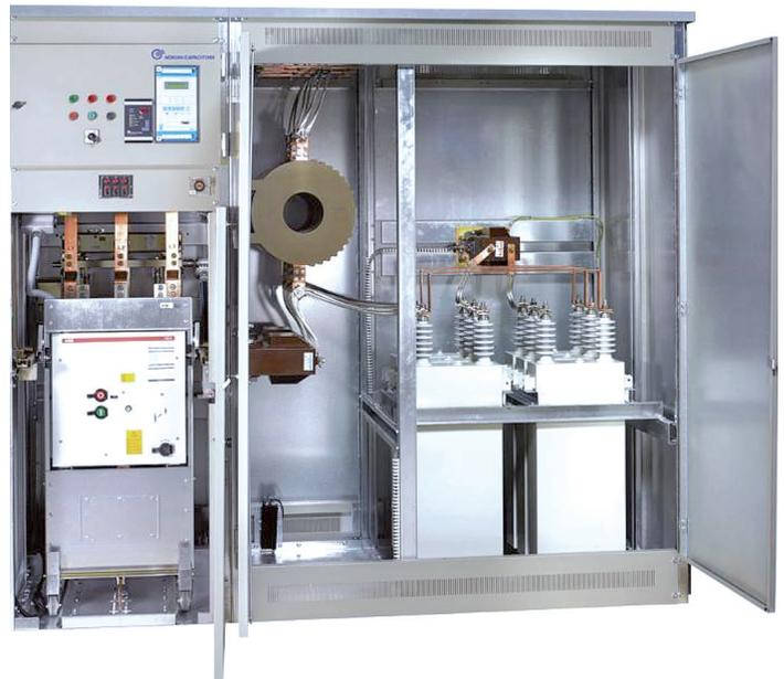
The construction of these banks is basically the same as the fixed banks, but they are fitted with a switching device (contactor or circuit breaker), that allows them to be connected and disconnected from the network at any time.
