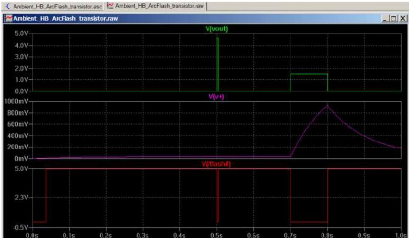
Figure 9. Arc Flash Heart-beat pulse and an Arc Flash Event
