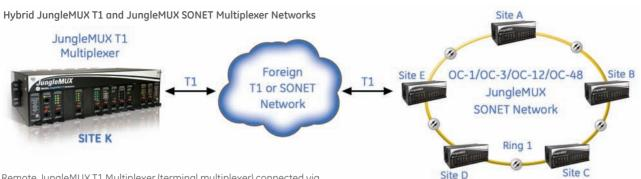
Remote JungleMUX T1 Multiplexer (terminal multiplexer) connected via a T1 link to a JungleMUX SONET network. DSO circuits from remote Site K are groomed into a T1 link for connection to Site E.
