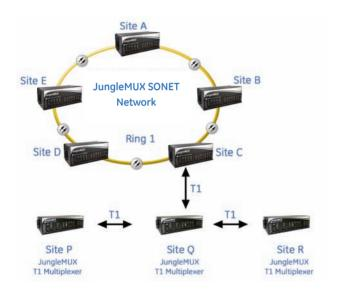
Remote JungleMUX T1 Multiplexers (Add/Drop) are connected to a JungleMUX SONET network over a T1 link. DS0 channels from Sites P and R are consolidated at Site Q and groomed for T1 connection to Site C
