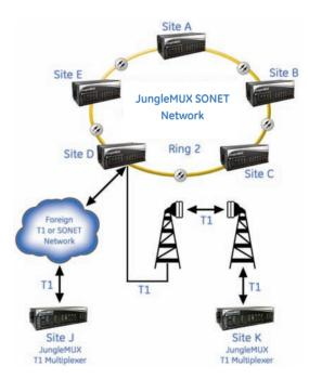
Remote JungleMUX T1 Multiplexers are installed at Site J and Site K. DSO channels from Site J and Site K are groomed and consolidated at Site D along with other DSO channels and transported in a SONET shared VT to another site, such as Site A.
