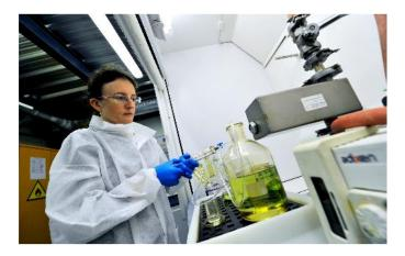
Oil samples are collected on site and analyzed by experts in our GE laboratories or by a local partner. Dissolved gas analysis on standard gases and complementary ones including oil quality, dielectric breakdown voltage, furans, moisture, and acidity can be performed. A report is generated that includes remedial actions and condition severity as per IEEE® or IEC® standards. Data can also be automatically transferred to the enterprise asset performance management system.
