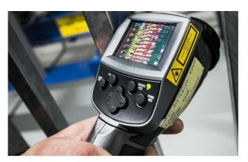
Hot spots generated by temperature increase due to electrical or insulation failure can be rapidly localized, even when the access is difficult. Therefore, remedial action of maintenance can be take before the equipment might be damaged.
