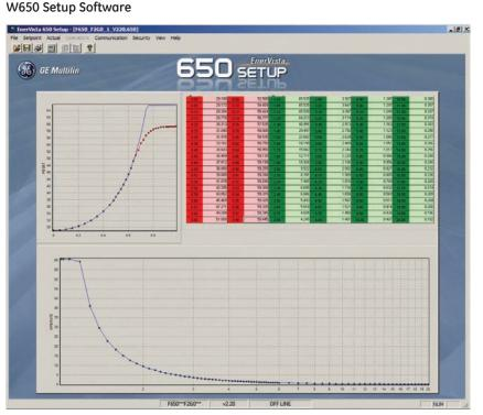
Create overcurrent curves customized to the characteristics of a wind generator using the W650 setup software
