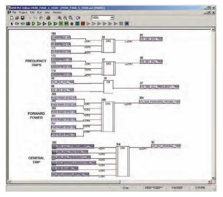
The W650 programmable control logic allows for the creation of customized wind generator protection schemes and applications.
