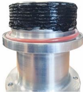
Figure 9-9: Bushing Adaptor with all threads covered in grease
