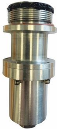
Figure 9-8: Bushing Adaptor with initial threads covered in grease
